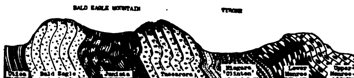
FIG. 1183. — Section of Bald Eagle Mountain, central Pennsylvania, a double ridge formed by the resistant sandstones and conglomerates with red beds between, each about 1000 feet thick. The Niagara is mostly represented by shales and sands, the lower Monroe by thin-bedded ribbon limestones, and the upper Monroe by a massive coral limestone (Lewiston limestone). (Original.)
